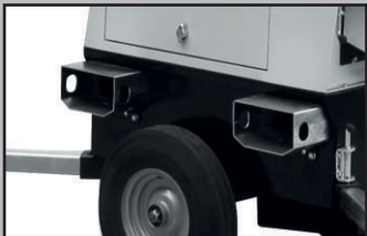
Large forklift pockets for easy loading and unloading.
